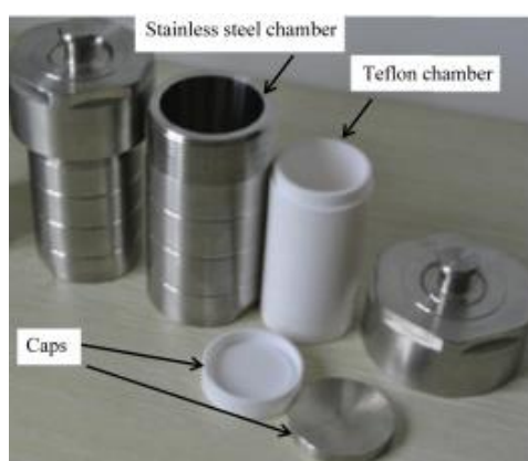
Figure 3-18: Breakdown of an autoclave (Kafle, 2019)
